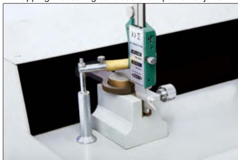
lapping measuring surfaces of caliper lower jaws
