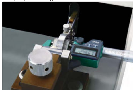
lapping measuring surfaces of outside micrometer
