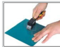
step 1: make grid cutting on surface
