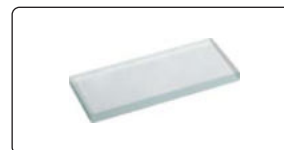
50mm reading scale (check magnification accuracy)
